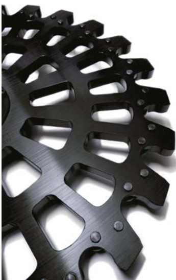
The indexed star wheel of an inspection machine receives articles from a conveyor and performs a rotate-and-stop cycle. Each time the wheel stops, static measuring heads perform one of a number of tests, checking parameters such as wall thickness (image: Heye International).
